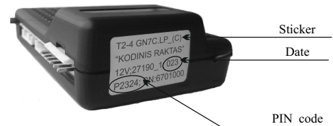
ne Pic. 1. Alarm System GN7C. The System Unit. Identification sticker, date and PIN code.
